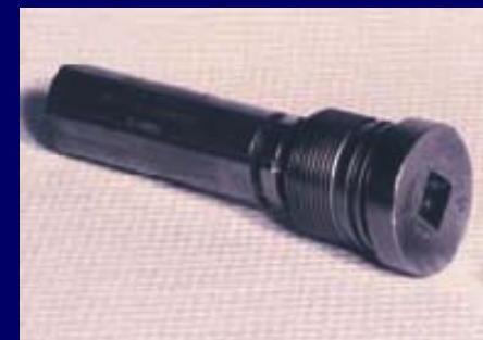
Am-241/Be neutron source for oil well logging
